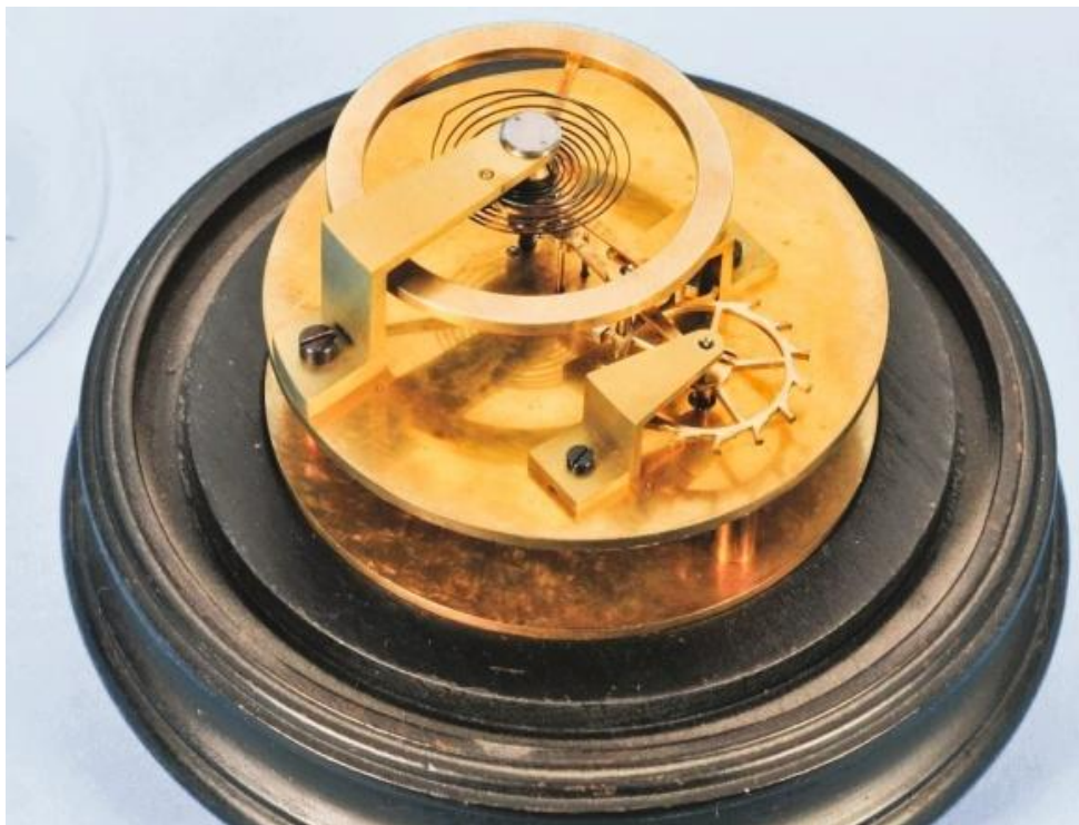
Fig. 14: Swiss anchor model signed 'Großmann Nr. 7349' [21].
