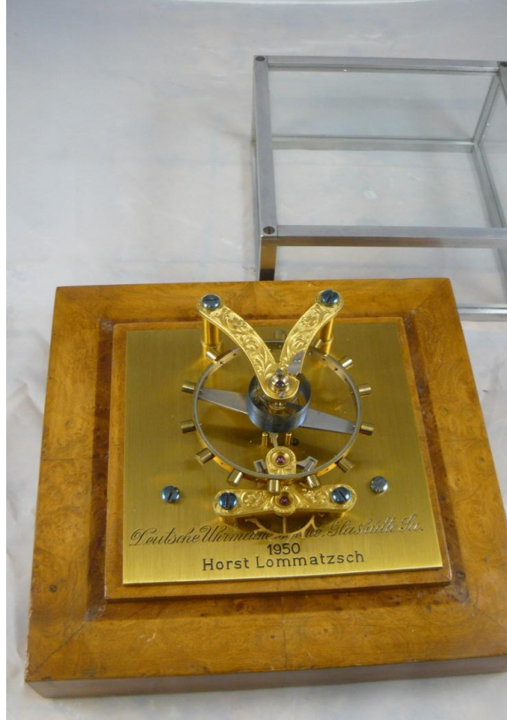
Fig. 15: A square design, very late (1950) Gangmodell of the Glashütte school by Horst Lommatzsch (school registry number 4358) [23].
