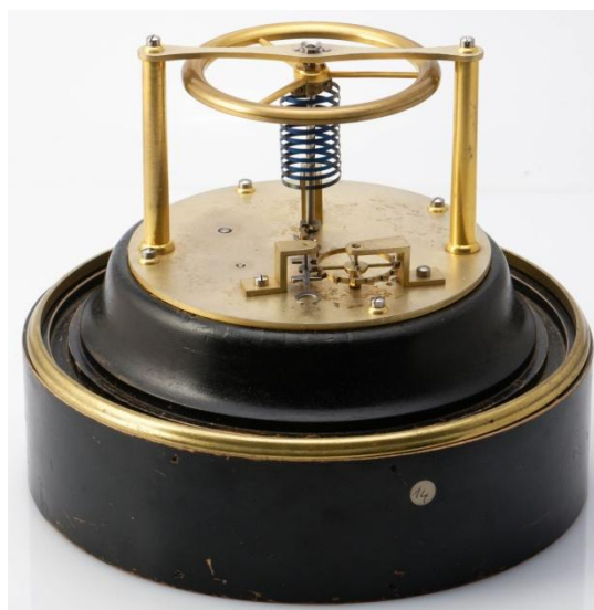
Fig. 12: Typical arrangement of the Cluses escapement models.
