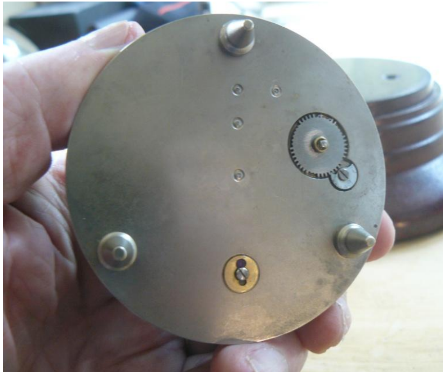
Fig. 5: Outside of bottom plate with (damaged) winding ratchet and click. The brass chaton holds a jewel supporting the balance wheel pivot.
