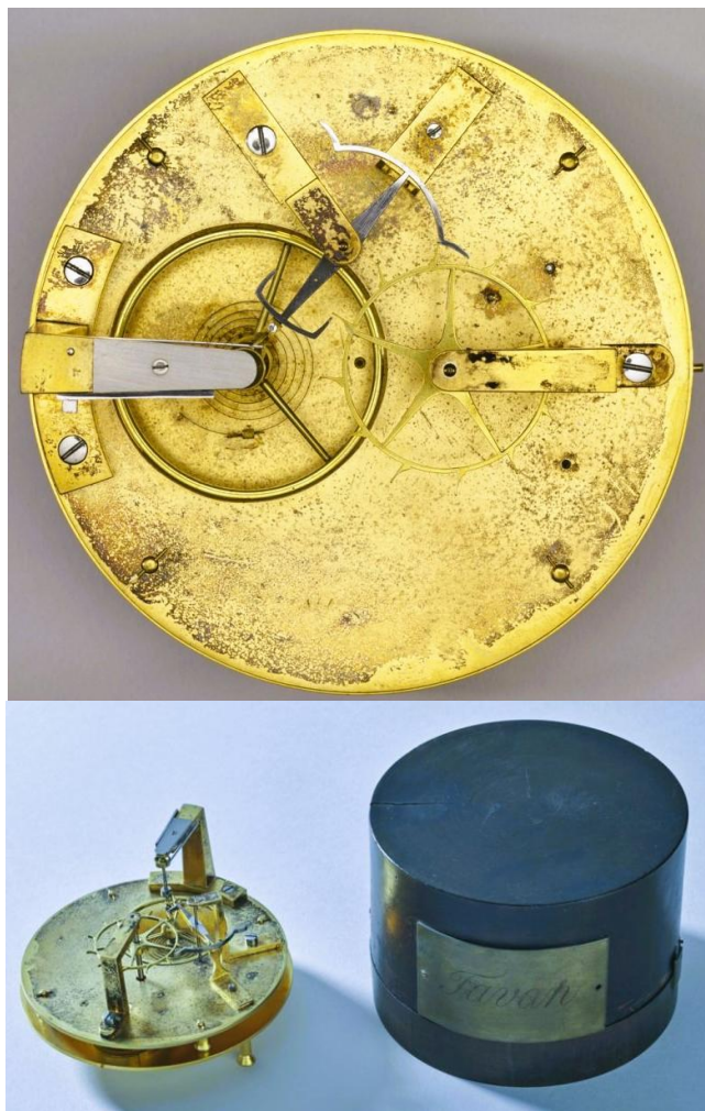
Fig. 11: A model of a curious form of anchor escapement made by Antoine Tavan in 1805. This is one of ten escapement models made by Tavan held in the Musée d'art et d'histoire Geneva. Inventory number AD 2550.
