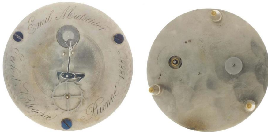
Fig. 7: A Bienne escapement model made by Emil Mutschler in 1888 [8].
