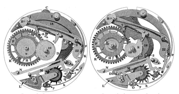
Figure 98 Stogden repeater at rest
