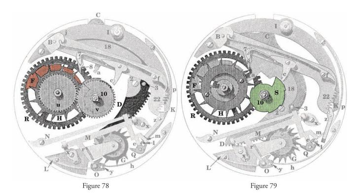
The hour-snail F (red) is a normal 12-step snail and requires a freedom mechanism for the change from XII to I hour. For it to function correctly the canon pinion must be placed on the center-wheel arbor and meshed with the intermediate-wheel R so that the hour and half-quarter snails are correctly aligned; as we will see later, this was not done correctly when the illustrations were drawn. Also, there must be minimal play in the gearing to avoid inaccurate striking.
