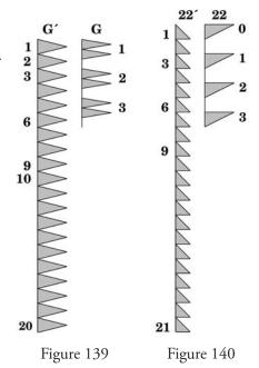
Immediately after striking the hours, the quarter-counting piece is raised, lifting the minute-counting piece with it by the gathering pallet r. So the hammer pallets are immediately raised above both strike racks and no quarters or minutes sound.
