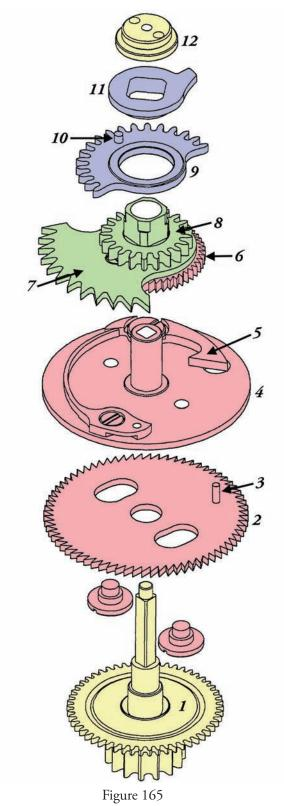
At this point the hour rack 7 is free and rotates clockwise until the sonnerie rack 13 (Figure 163) has dropped onto the hour-snail. The gathering pallet 11 rotates with it, allowing the quarter rack 14 and minute rack 15 (Figure 164) to drop onto their respective snails, and the train lock lever 16 releases the small train.
