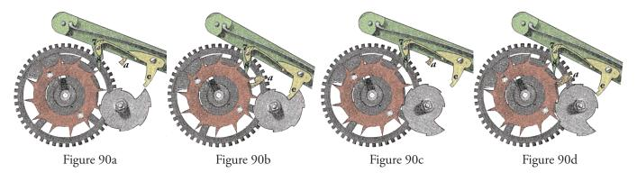
This applies to all hour changes, including from XII to I. But the XII to I change requires freedom between the leading edge of the hour-snail arm and the side of the I hour step to avoid stopping the canon pinion. So the XII hour step is made wider, and the I hour step narrower to provide this freedom, while the advance of the hour-snail on the hour ensures correct striking.
