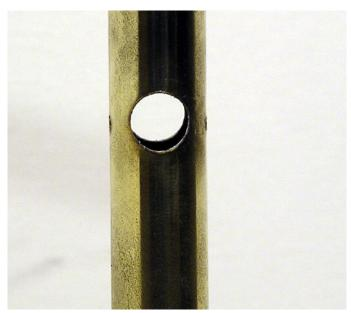
Cut the ends of the pin leaving about 1mm to round
