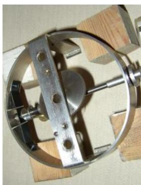
Remove the barrel and service the clock in the same way as any other Atmos. Make sure you check the poise of the pallets and fork assembly. Mine was off and I had to take it apart again!
