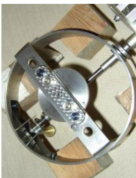
Support the frame safely on four 60mm blocks.
