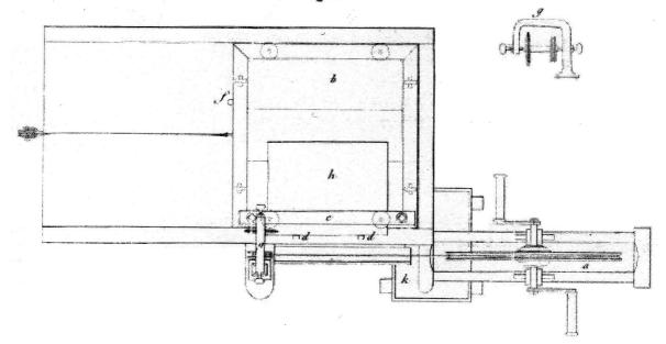
**Figures 3**, and 4: Elevation, plan and details of the lathe used to turn plates; like the turns with a bow, it is fixed in a vice or on a bench as required.
