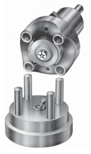
Punch and die to cut out wheels, tool designed by P.-F Ingold.
