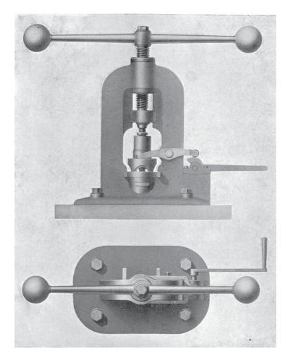
Press to cut out wheels (reproduction of a drawing by Ingold).
