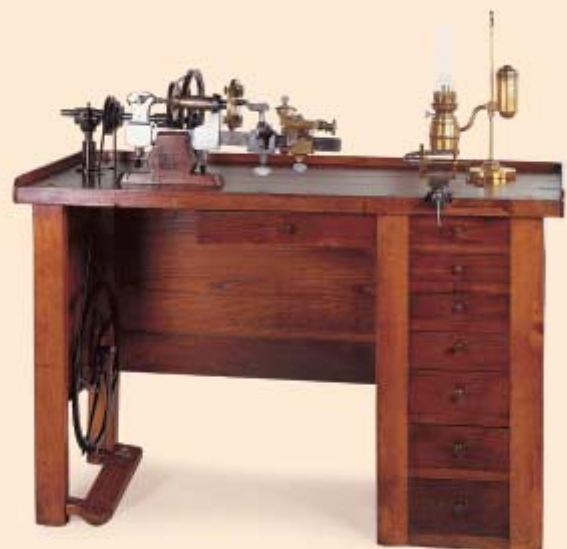
watchmaking bench equipped with face plate engine
