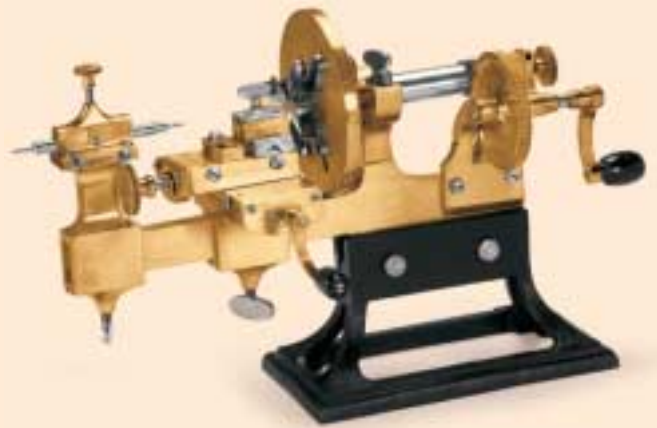
brass face plate engine
