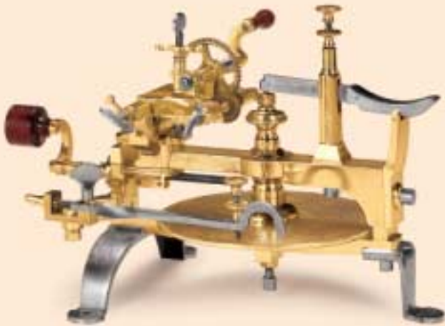
wheel dividing engine
