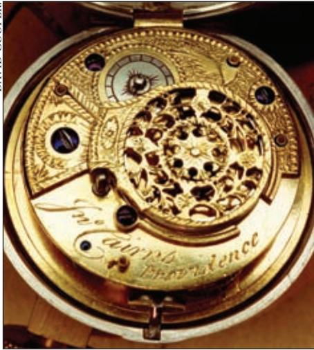
**Figure 13.** John Cairns, Providence. Earliest documented example of an American-made watch, and subject of an extensive article by David Cooper in the February 2002 *NAWCC Bulletin*, evidencing locally made components and assembly, ca. 1790. Verge fusee movement with enamel dial, gold hands, and fully pierced balance cock signed John Cairns, Providence.
