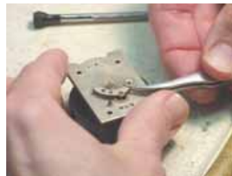
Fig. 21 Lifting escape wheel bridge straight up
