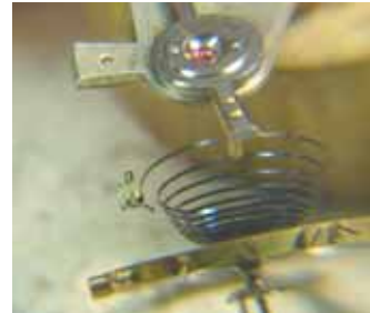
Fig. 19 Hairspring stud freed from balance bridge
