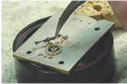
Fig. 38 Positioning escape wheel and fork
