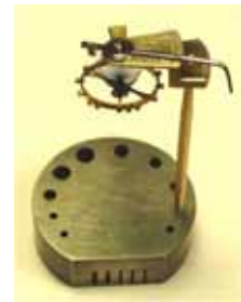
Fig. 48 Balance on balance tack for beat adjustment
