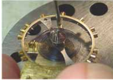
Fig. 43 Rotating regulator boot to capture hairspring
