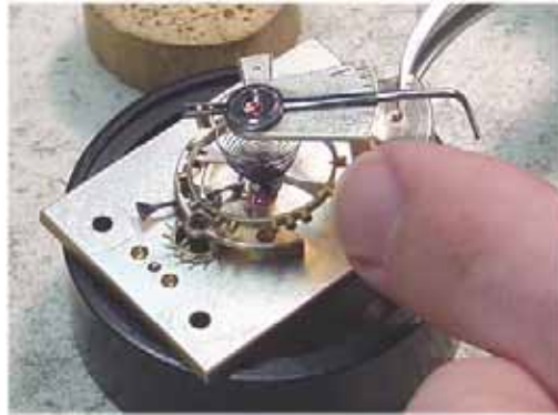
Fig. 45 Assembling balance bridge to platform
