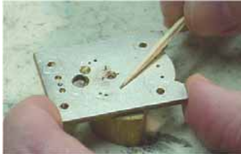
Fig. 28 Polishing the plates with the toothpick rub
