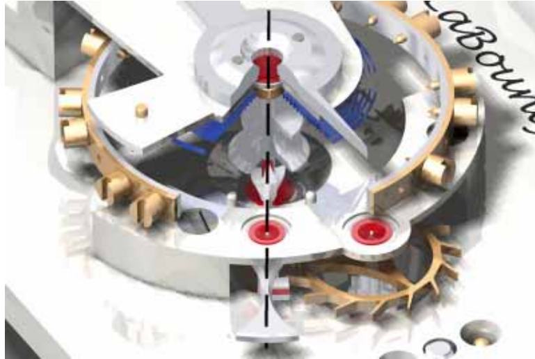
Fig. 49 Setting the beat using a sight reference (shown cut-away for clarity)
