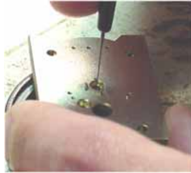
Fig. 37 Oiling lower balance jewel
