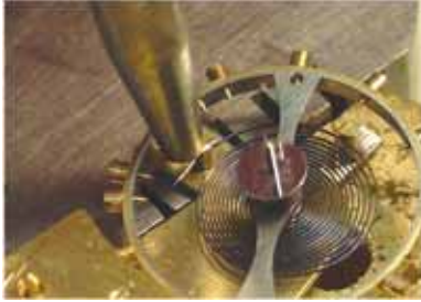
Fig. 42 Pressing in hairspring stud
