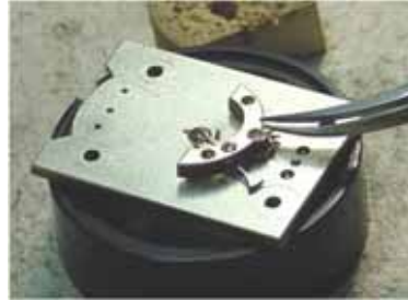
Fig. 39 Assembling escape wheel bridge
