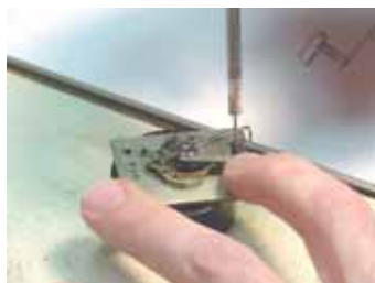
Fig. 15 Removing the balance bridge
