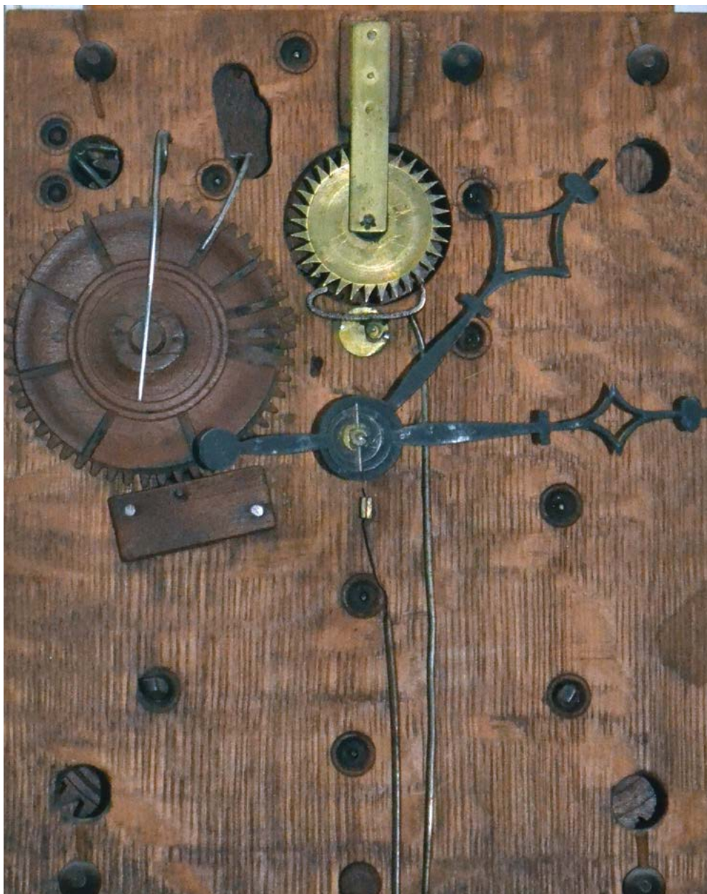
Figure 2. Eli Terry's 5-arbor wooden movement with count wheel.
